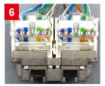
Repeat the connecting with the remaining wire pairs according to Figures 4 and 5. Visually check the single sliders for correct contact.
