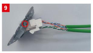
Insert the module into the side guides of the adapter and press it in. At the end of the process, the module snaps into the adapter with a "click".
